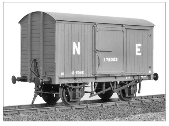
**PROTOTYPE.** Several thousand of these 10ft wheelbase, vacuum brake fitted, wooden underframe versions of the LNER's standard van were built from 1934 onwards. They lasted well into British Railways days and worked all over the country. They were XP rated and so could run in local passenger trains and one of these vans tacked onto the rear of a sleepy branch line local to convey urgent traffic to the junction would be a common sight.
